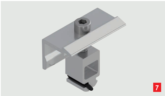
Universal end clip with cylinder head screw M8 for module heights of 30–40 mm or 41–46 mm
