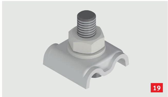
Lightning protection terminal block for 8 mm lightning protection wire, pre-assembled with hammer-head bolt
