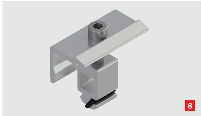
Universal end clip with cylinder head screw M8 for module heights of 30–40 mm or 41–46 mm for start support and double support
